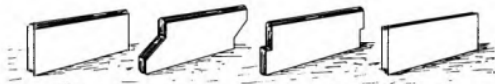
Above: Examples of concrete staves, circa 1919. 56 Below: Detail of south elevation of north silo showing its concrete stave and steel reinforcement hoop construction.
