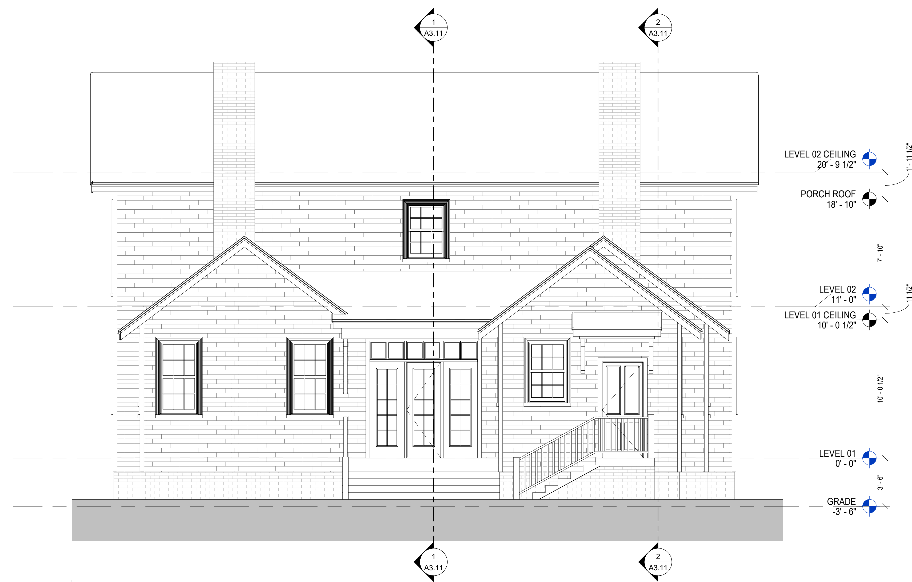
2 BUILDING ELEVATION - NORTH A3.02 1/4" = 1'-0"
