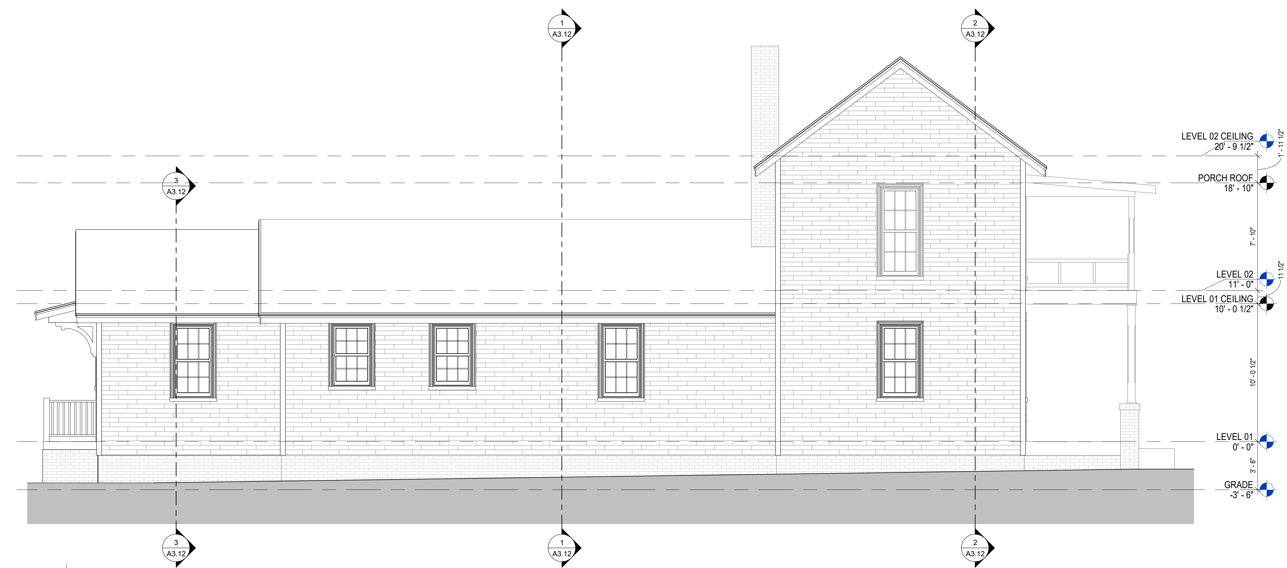
1 BUILDING ELEVATION - WEST A3.02 1/4" = 1'-0"
