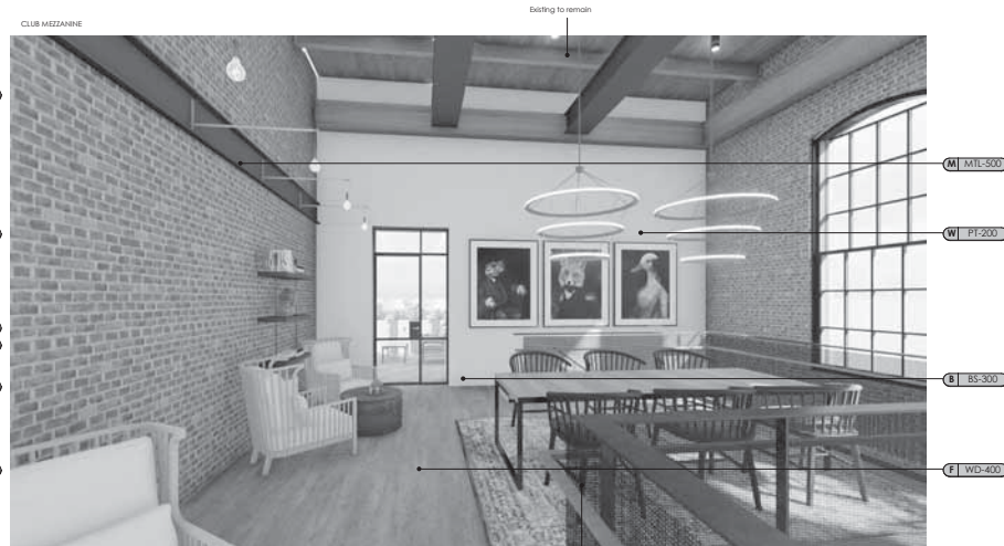
Perforated metal railing with matte black guardrail and stained wood handrail.
