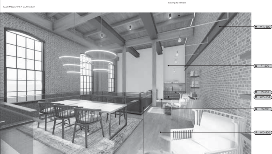
Perforated metal railing with matte black guardrail and stained wood handrail.
