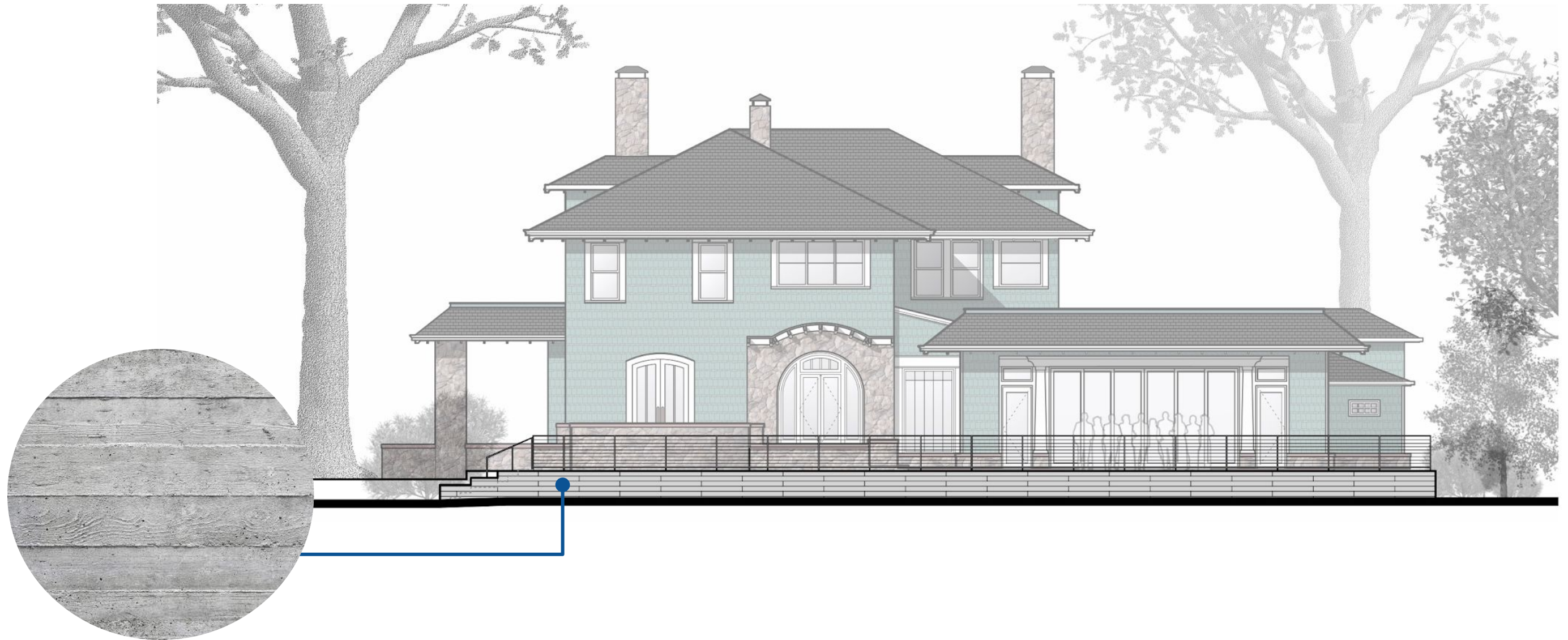
Board Formed Cast-In-Place Concrete Retaining Wall
