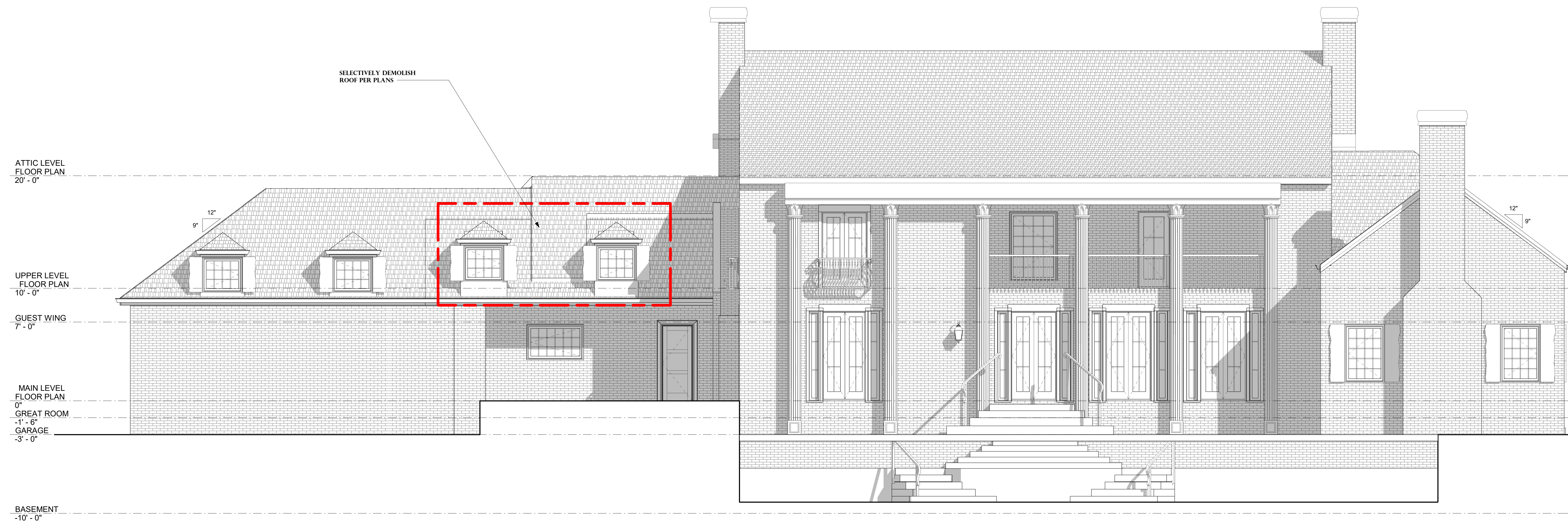
① REAR ELEVATION - EXISTING/DEMOLITION 1/4" = 1'-0"
