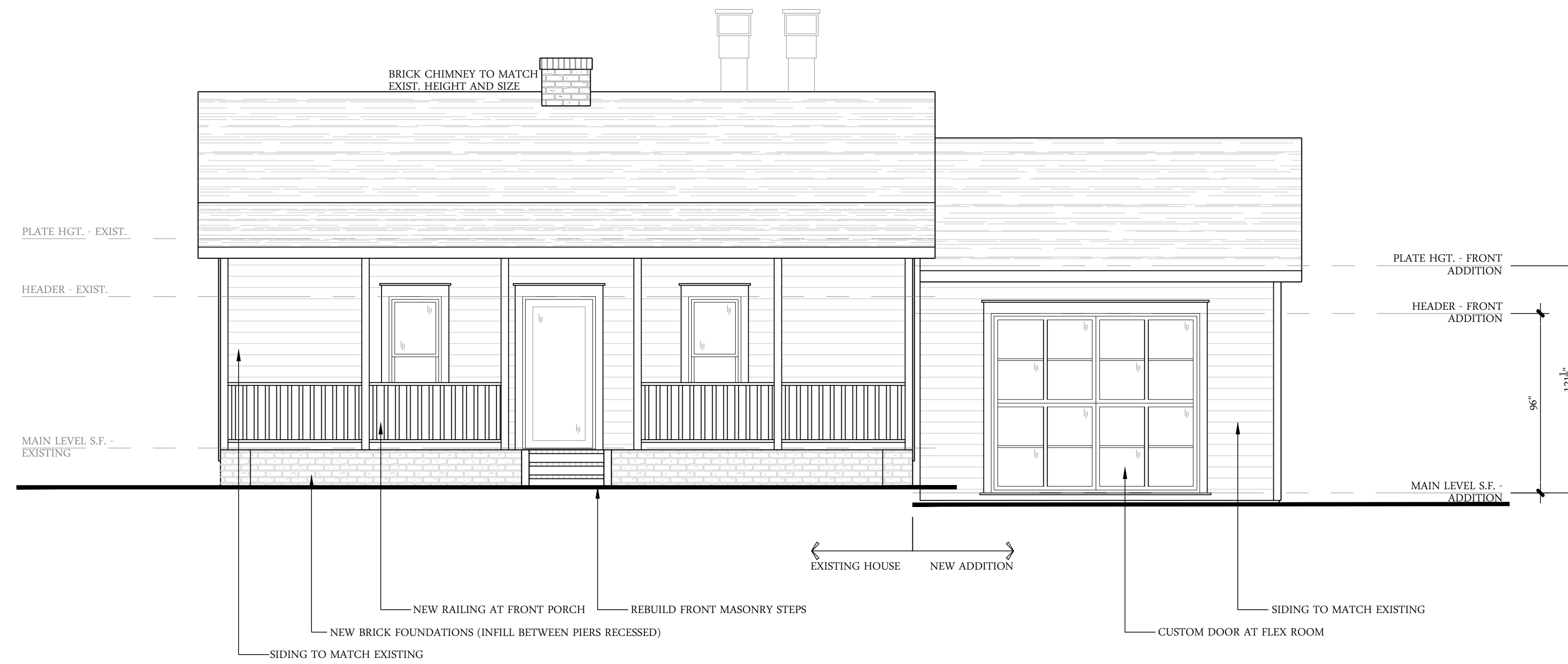
1 NEW FRONT ELEVATION (DELBURG STREET) 1/4"=1'-0"
