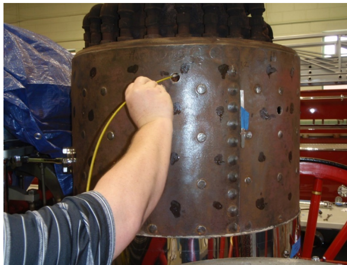
Boiler Tests To Certify "Old Sue."
