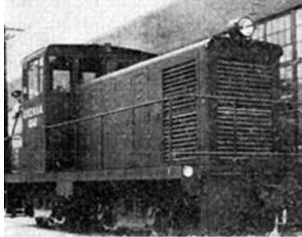
*Diesel-Electric GMC Locomotive used to Move
